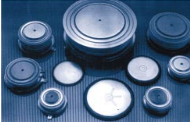
Figure 5 High power semiconductors. The sizes of these chips as well as the power density increase, allowing for the switching of tremendous powers.
